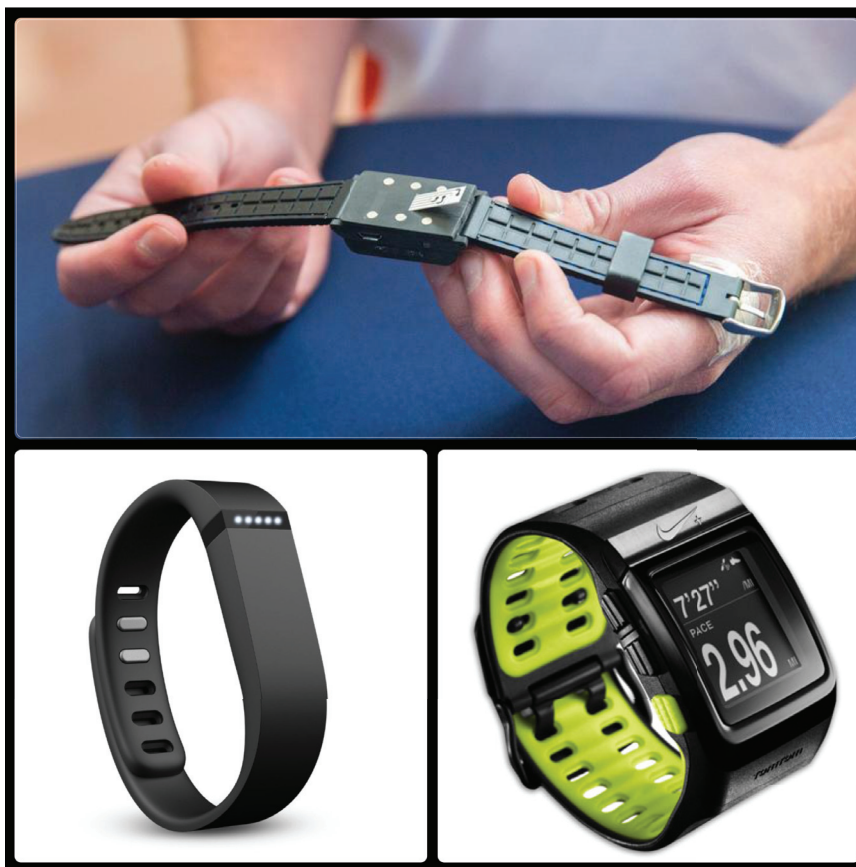
Figure 4.1: This figure highlights the accessibility challenges in two wearable fitness trackers currently on the market. The electrozyme watch (top) measures enzymes in sweat, which may not be effective for some users with spinal cord injury. The Fitbit charge (left) is used as a step counter, which is not a useful measurement for wheelchair users who don't walk. The clasp used on the Nike+ GPS Watch (right) can be difficult for users with limited hand dexterity to use independently.
